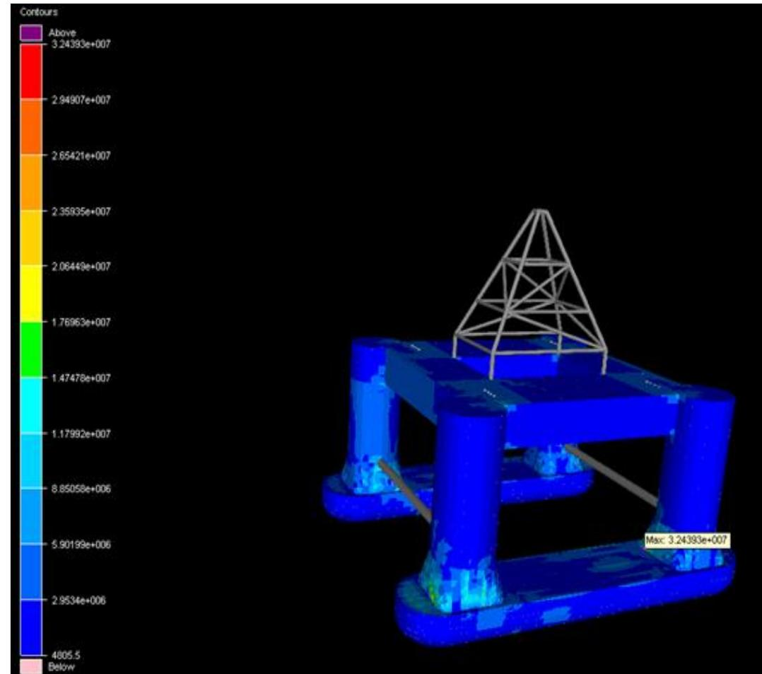
**Critical Location: Pontoon-column connection (Max.Von-Mises Stress)**
